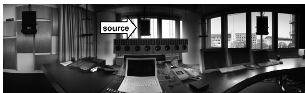
Figure 12: Listening test environment with the reference loudspeaker from the perspective of the listener
